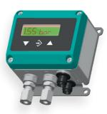
ΔP measuring by calculating the difference between two Pressure sensors
